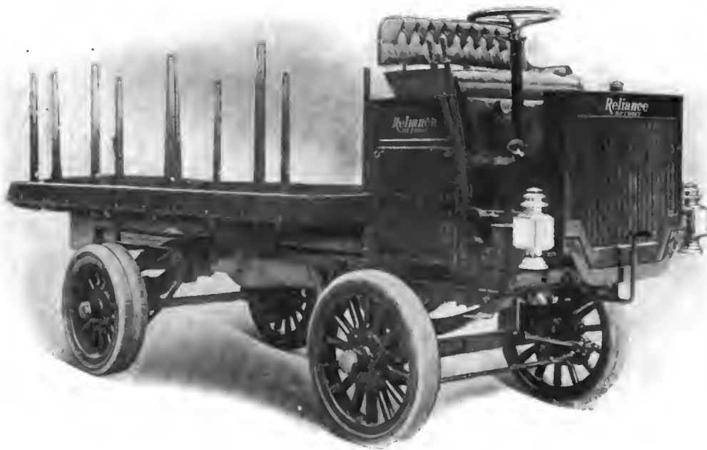
RELIANCE OPEN DELIVERY VEHICLE, TWO-CYCLE, 4 CYLINDERS, 60-H.P., PRICE $4,400. Reliance Motor Car Co., Detroit, Mich.
